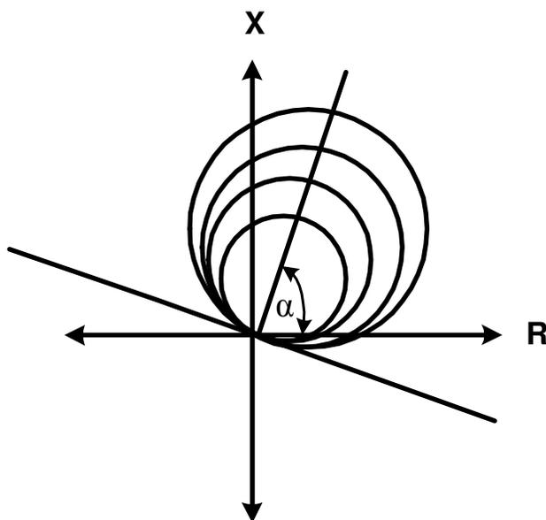
**Figure 25: Four Stages Mho Distance Relay**
