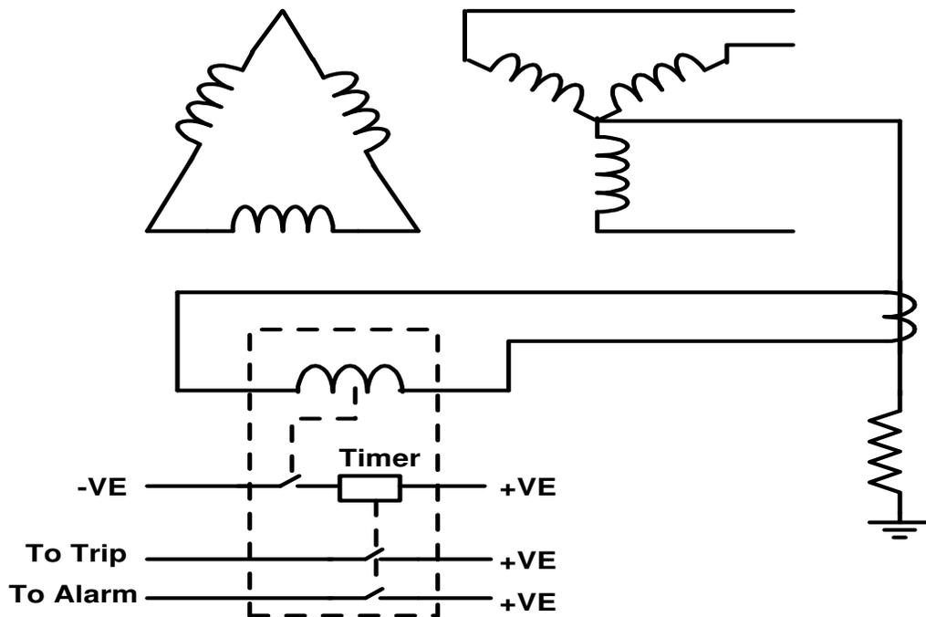
Figure 17: Earth Fault Relay connected Star Point of Power Transformer
