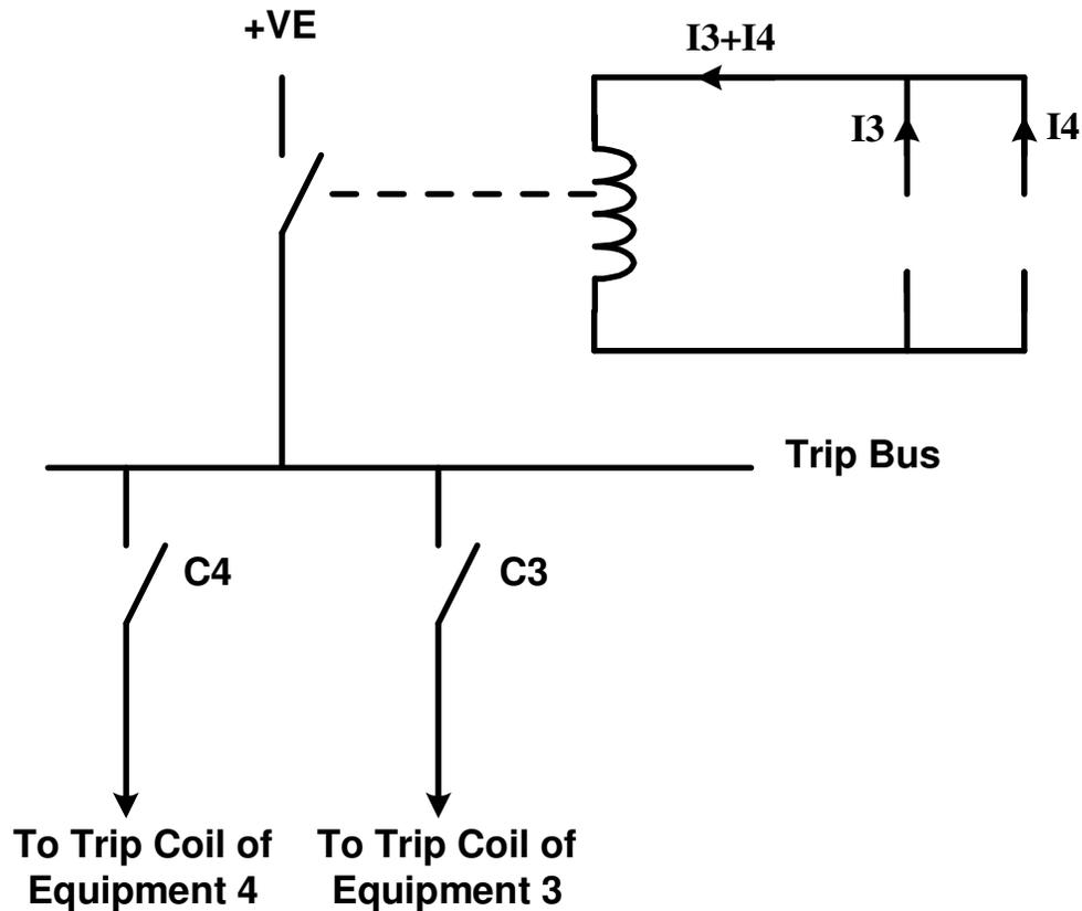
**Figure 54: Tripping Circuit of Bus Bar Protection**
