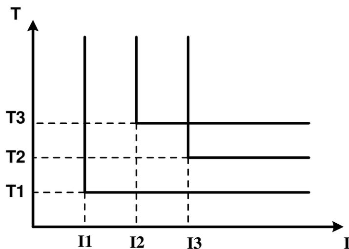
**Figure 11 Tripping Characteristics of Multi-Stage Definite Time Over Current Relay**
