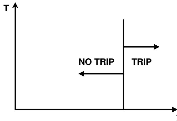
**Figure 9: Tripping Characteristics of Instantaneous Over Current Relay**
