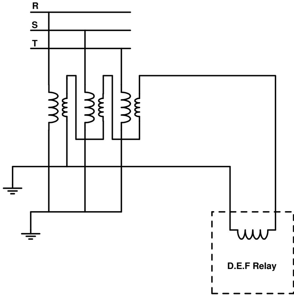
**Figure 6: Open Delta Connection of Voltage Transformer**
