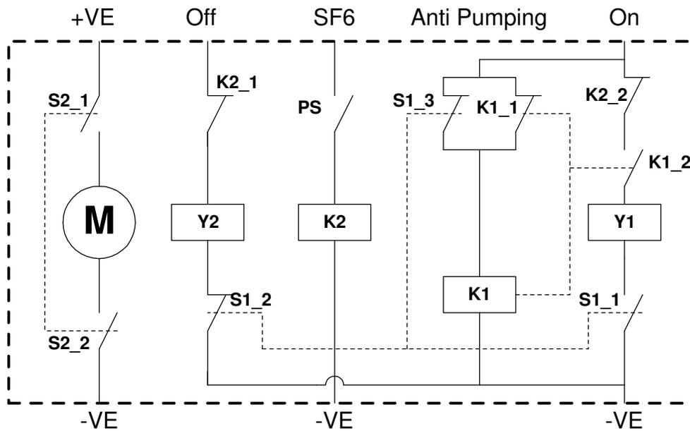
**Figure 62: Anti Pumping Relay while the Circuit Breaker is ON**
