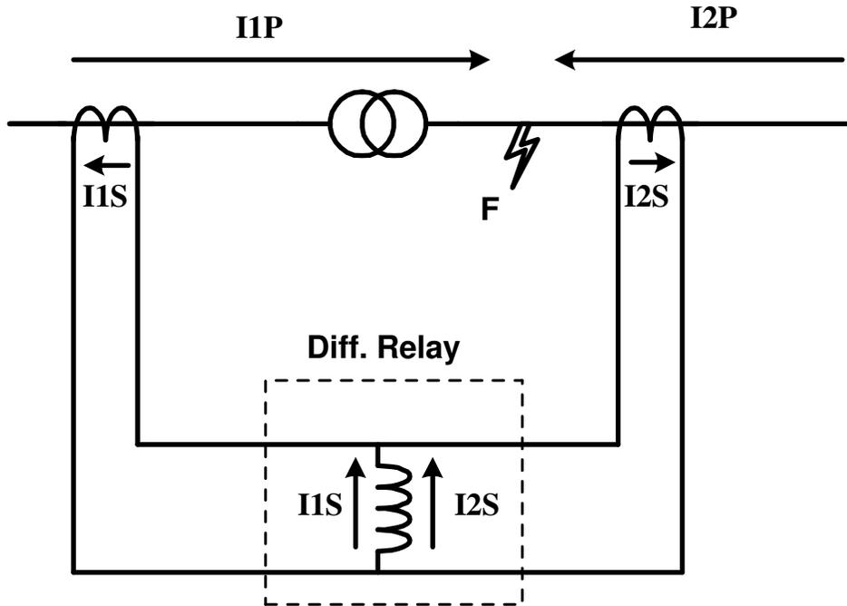
**Figure 37: Differential Relay at Internal Fault**
