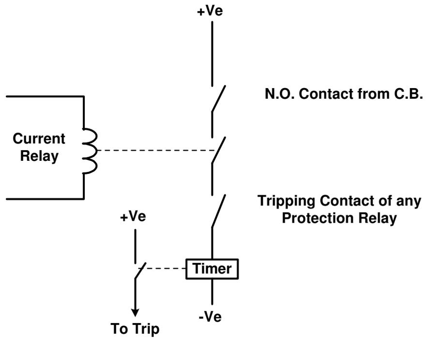
**Figure 55: Wiring Diagram Of Breaker Failure Circuit**
