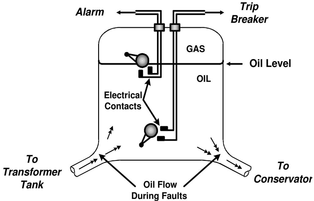
**Figure 46: Schematic Diagram of a Buchholz Relay Arrangement**
