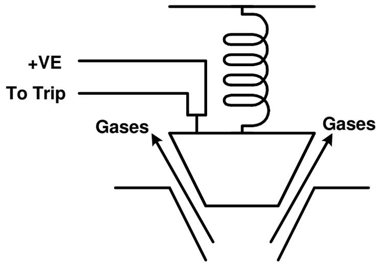
**Figure 49: Pressure Relief Durring Fault**
