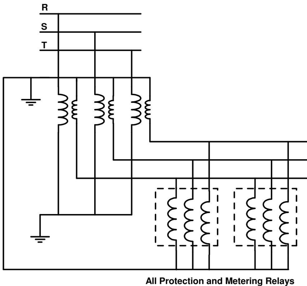
Figure 5: Star Connection of Voltage Transformer
