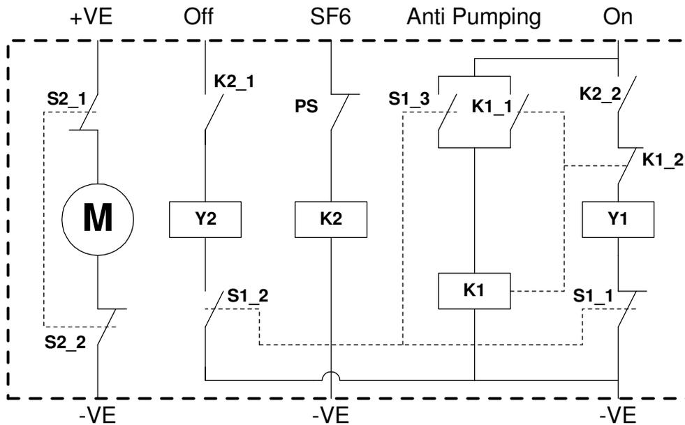
**Figure 57: Case1(Spring Uncharged and Gas Pressure Insufficient)**
