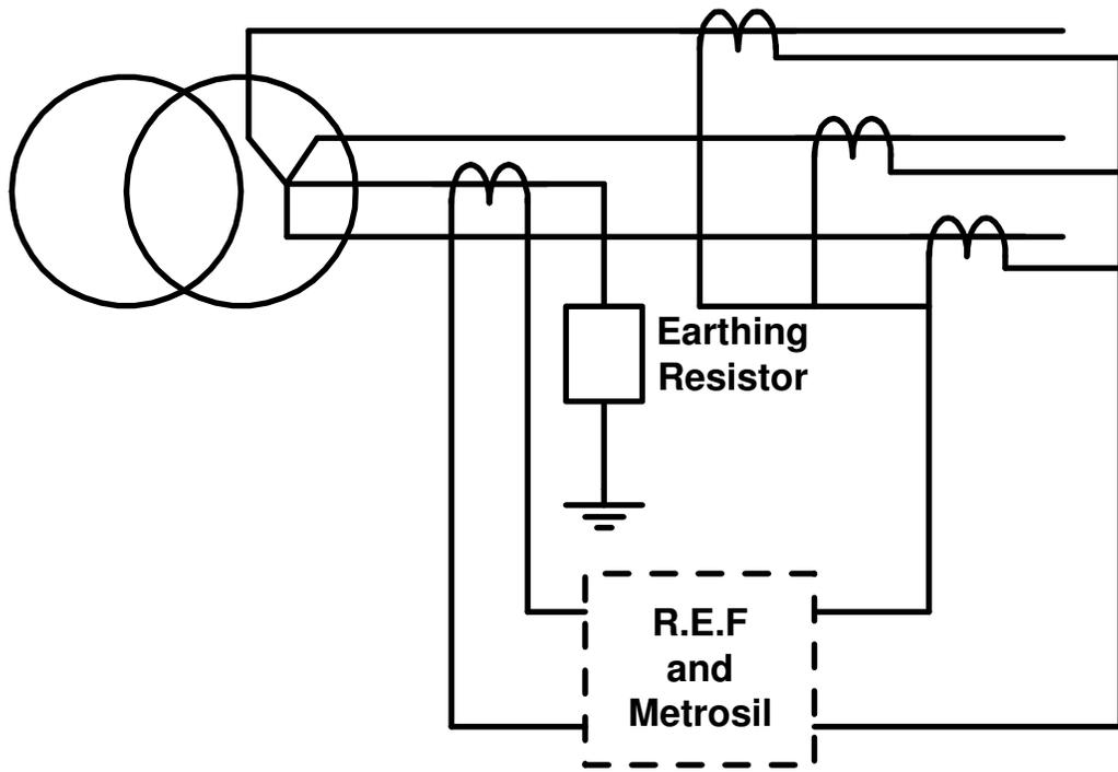
**Figure 43: Restricted Earth Fault Relay**
