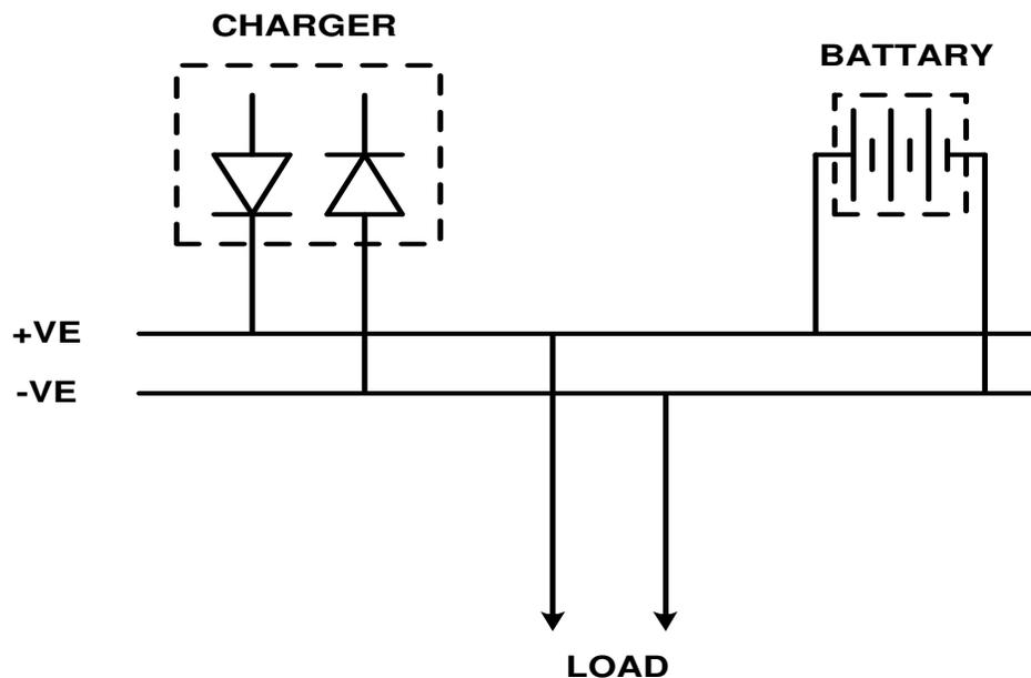
**Figure 7: DC System of a Substation**
