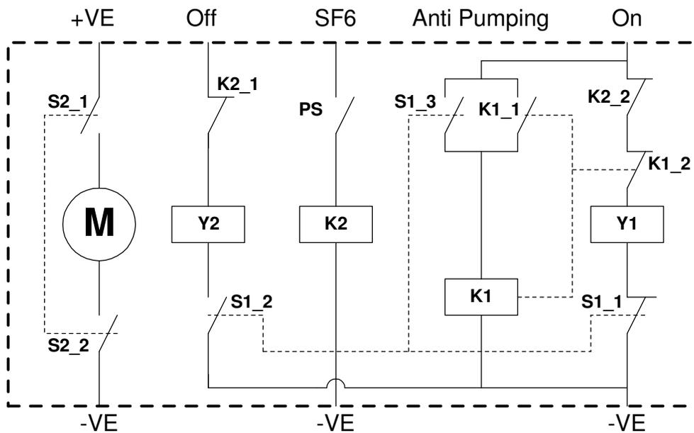
**Figure 59: Case3(Spring Charged and Gas Pressure Sufficient)**
