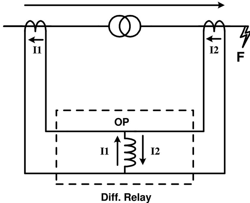
**Figure 36: Differential Relay at External Fault**
