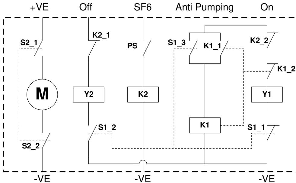
**Figure 56: Original Situation of Circuit Breaker**
