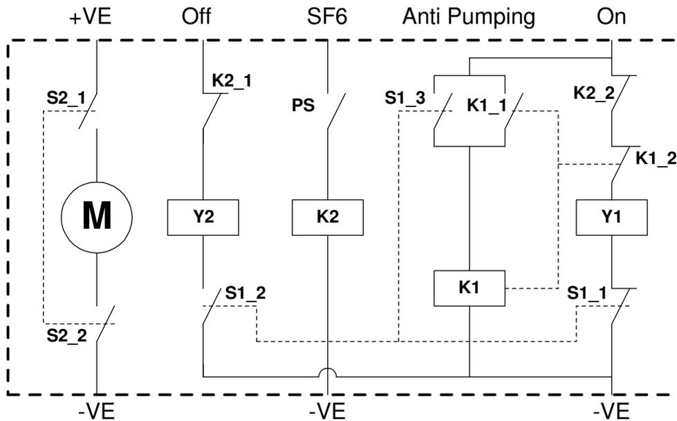
**Figure 61: Case5 (Circuit Breaker OFF)**
