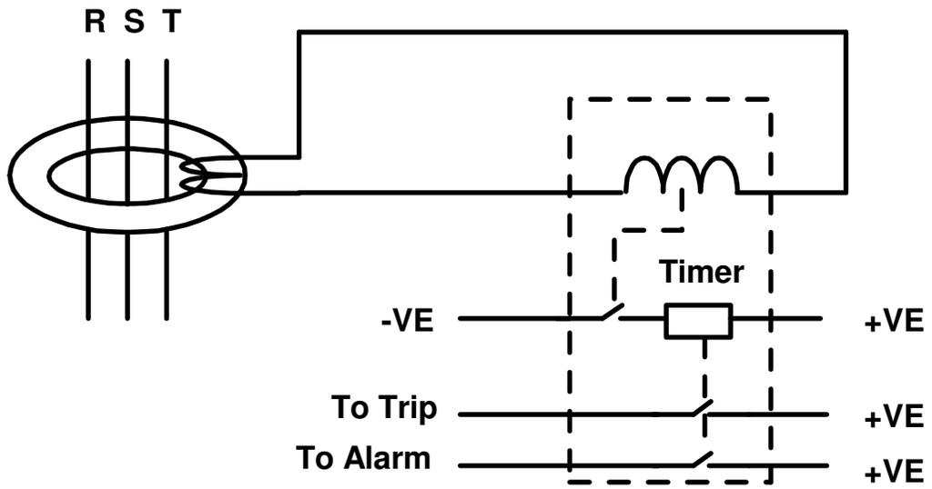
**Figure18: Earth Fault Relay connected to Ring Type Current Transformer**
