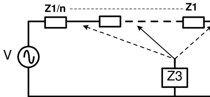
**Figure 21: Different Faults at Different Locations**
