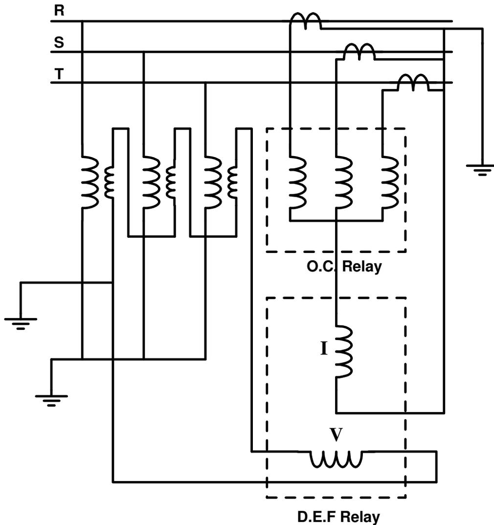
Figure 19 : Connection Diagram of Directional Earth Fault Relay
