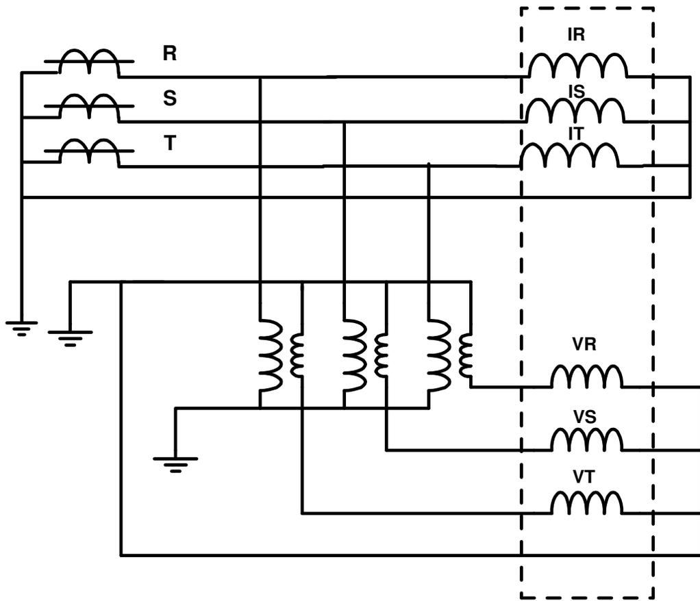
**Figure 15: Connection Diagram of Directional Over Current Relay**
