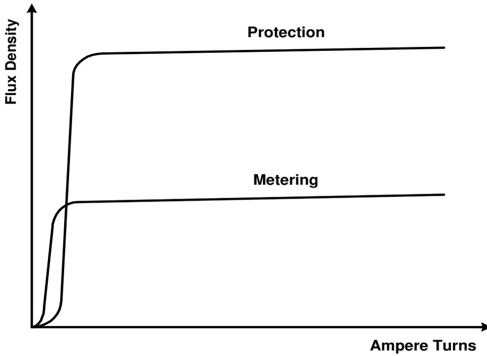
Figure 3: Protection and Metering Cores
