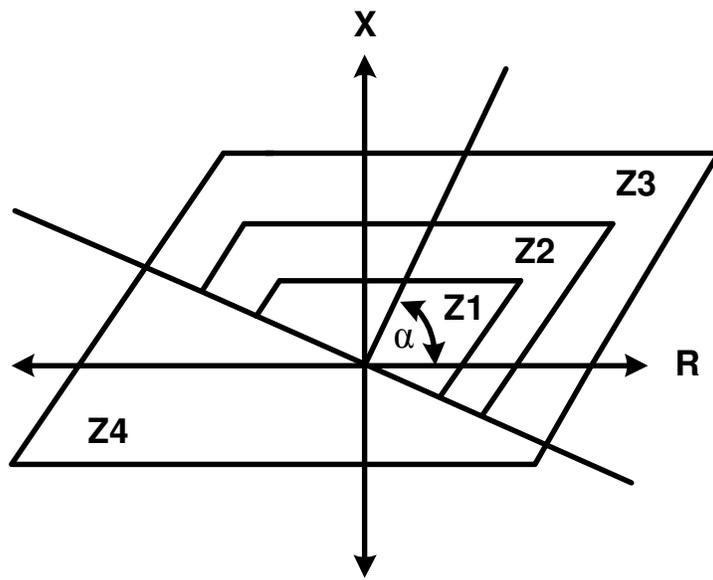
**Figure 26: Four Stages Quadrilateral Characteristics Distance Relay**
