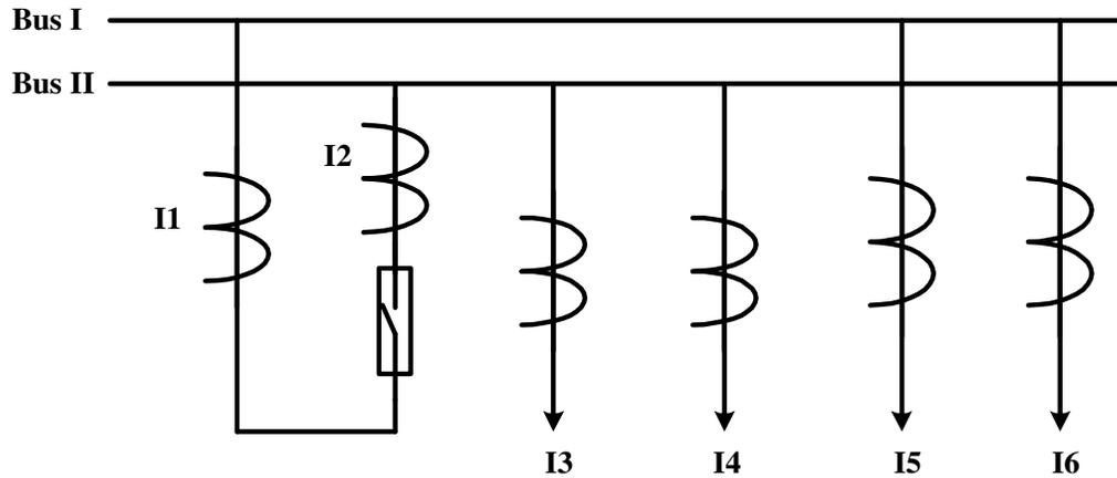
Figure 53: Simple Two Bus Bar System
