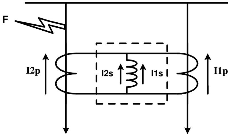
**Figure 52: Bus Bar Protection Relay at Internal Fault**
