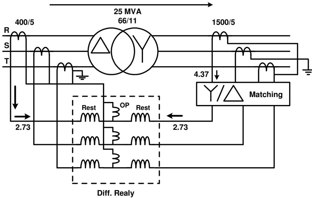
**Figure 39: Practical Example of Differential Relay**
