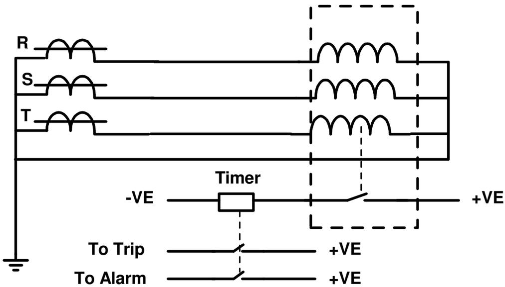
**Figure 13: Definite Time Over Current Relay with External Timer**
