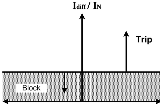
**Figure 40 : Tripping Characteristics of Simple Differential Relay**
