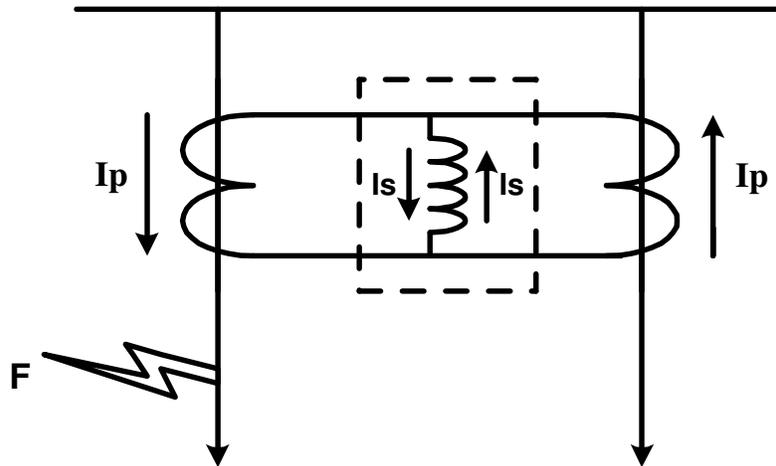
Figure 51: Bus Bar Protection Relay at External Fault
