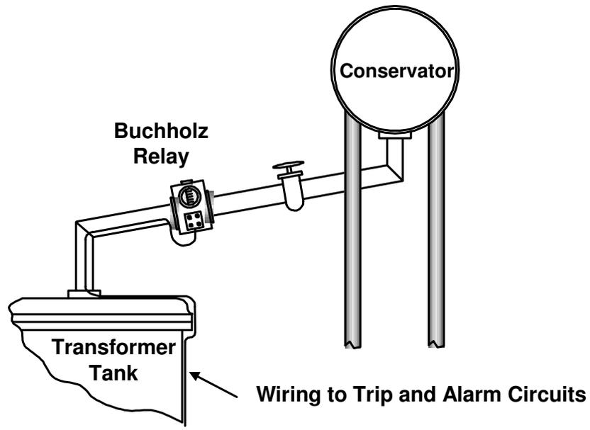
**Figure 45: Location of the buchholz relay on the transformer**
