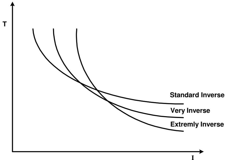
**Figure 14: Tripping Characteristics of Inverse Time Over Current Relays**
