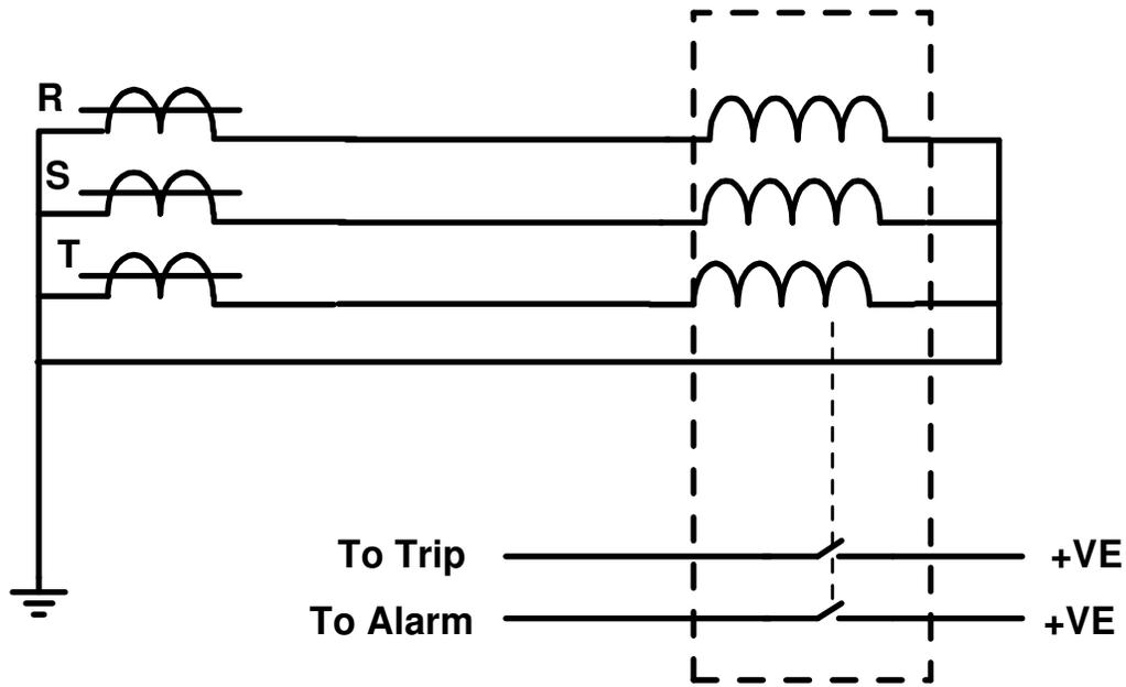
**Figure 10: Connection Diagram of Instantaneous Over Current Relays**
