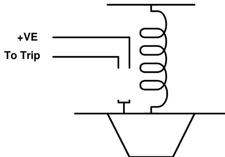
**Figure 48: Pressure Relief Before Fault Occurrence**
