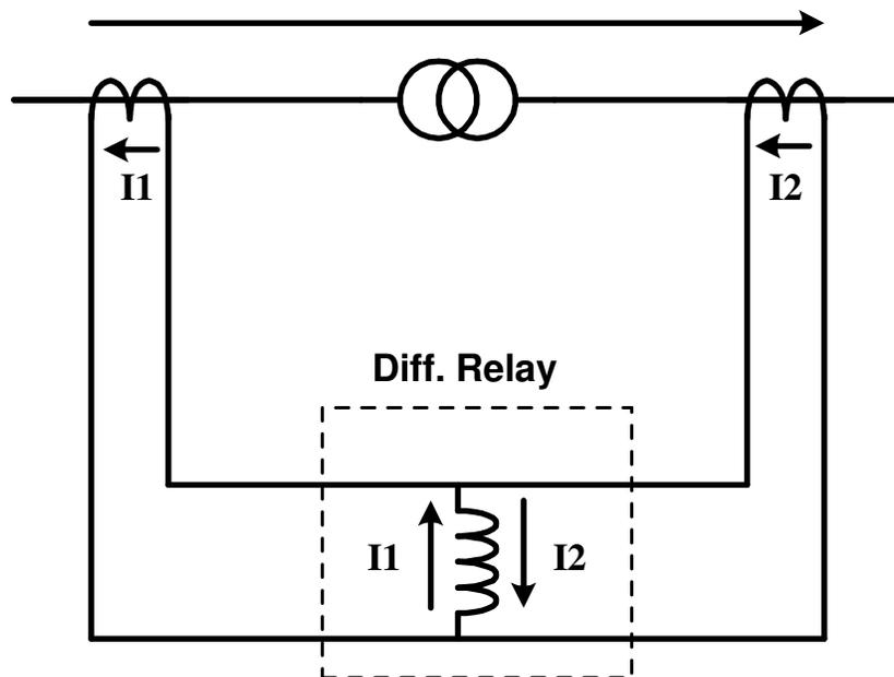
Figure 35: Differential Relay at Healthy Transformer
