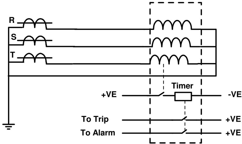
Figure 12: Definite Time Over Current Relay with Internal Timer
