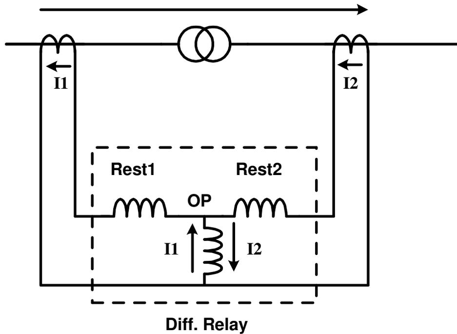
**Figure 38: Biased Differential Relay**
