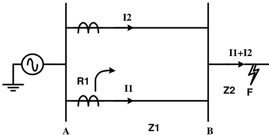
**Figure 27: Under Reach of Distance Relay**
