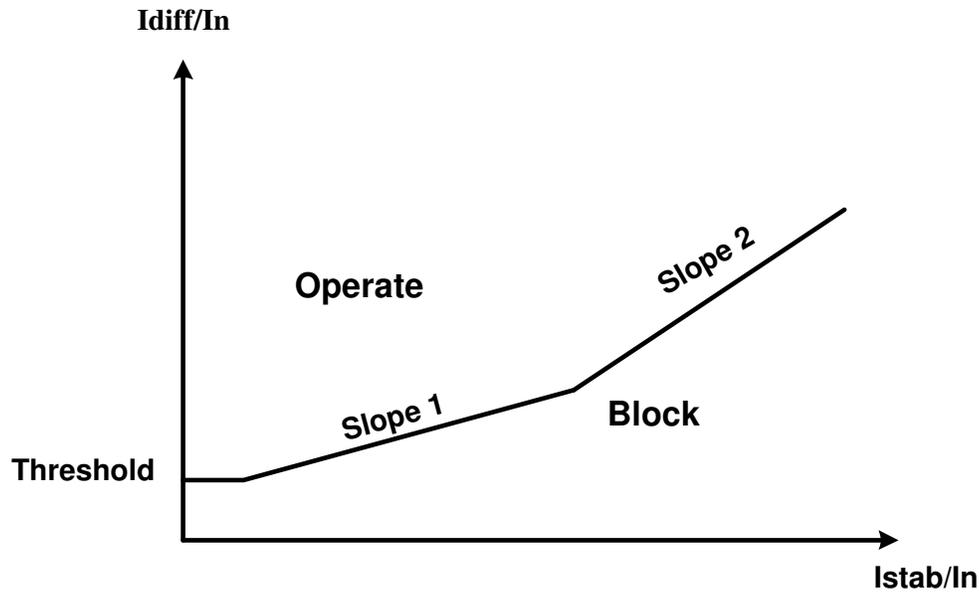
**Figure 41 : Tripping Characteristics of Biased Differential Relay with Two Stages (Two Slops)**
