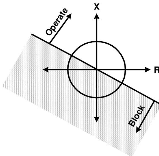
**Figure 23: Operate and Block Regions of Directional Impedance Relay**
