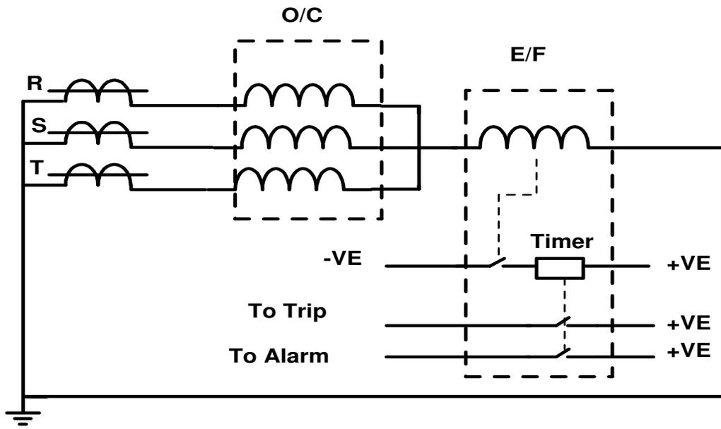
Figure 16: Earth Fault Relay connected at The Neutral Point of Current Transformer
