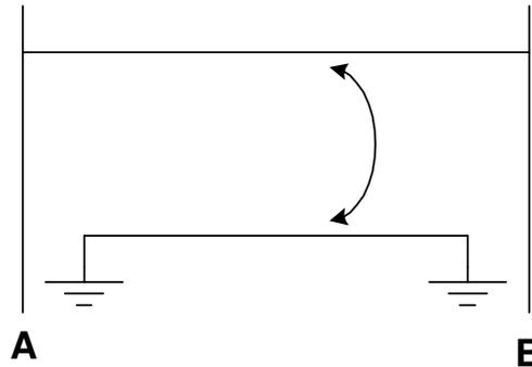
**Figure 28: Over Reach of Distance Relay**
