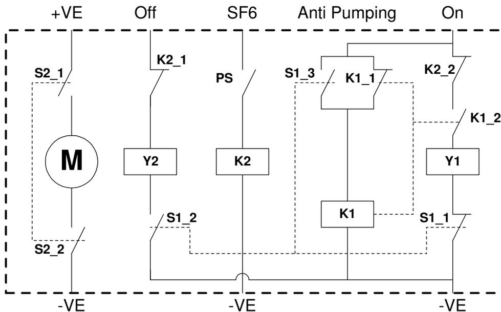
**Figure 63: Anti Pumping Relay while the Circuit Breaker is OFF**
