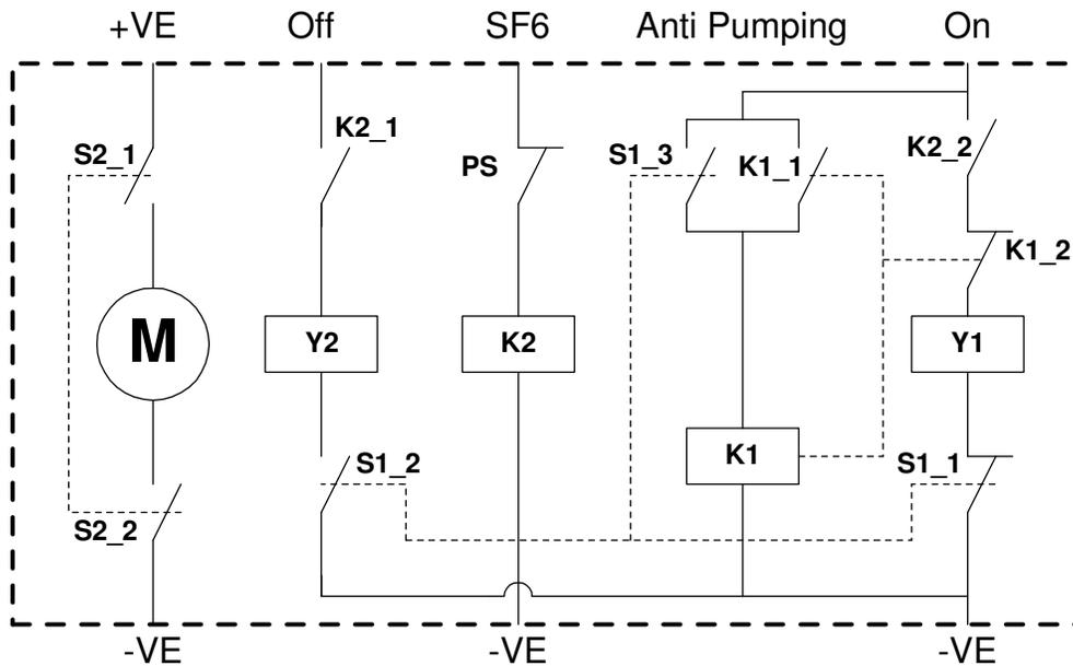
**Figure 58: Case2 (Spring Charged and Gas Pressure Insufficient)**
