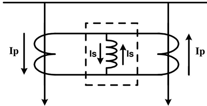
**Figure 50: Simple Bus Bar Protection Relay with Two Equipments**
